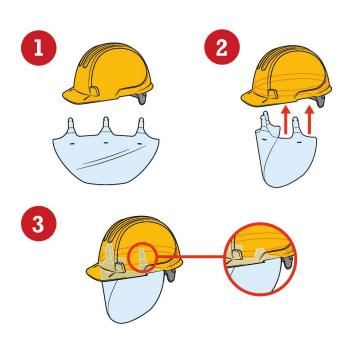
\*Bend armature around internal strap of the hard hat and insert hook into the slot in the visor
